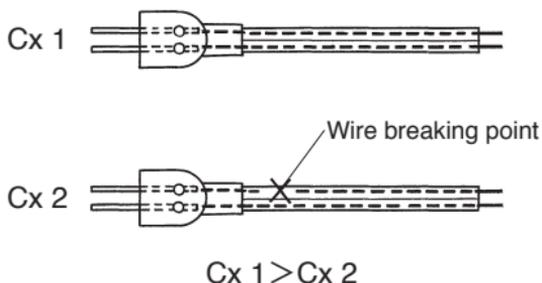
Continuity or open-wire check of parallel cords, as shown in Fig, can be done by measuring capacitance between the core wires (conductors) as a comparison test.
