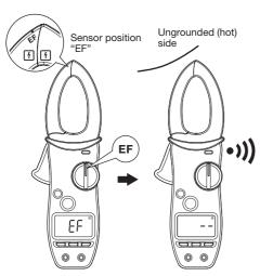
Bring the "EF" marking on the CT close to or in contact with the object to be measured. When the sensor is brought to the ungrounded (hot) side, "-" is displayed in front of the digits in the display, the buzzer sounds, and the EF detection LED flickers. On the grounded side, "EF" remains displayed and the buzzer does not sound. The higher the voltage to be detected, the larger the "-" digits in the display. The rate of intermittent activation of the buzzer and LED will also increase.
