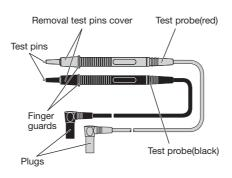
In case of test pins cover attached: CAT.IV 600 V. CAT.III 1000 V In case of test pins cover removed: **CAT.II 1000 V**
