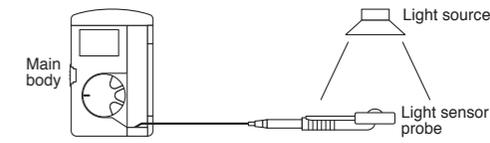
It is also possible to measure illuminance while the light sensor probe is integrated with the main body.
